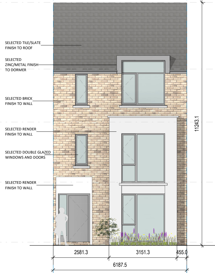
① H08 Brick Front Elevation (MT) 1 : 100
